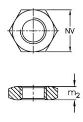
$\begin{array}{ll} m2 &= 13.5\\ Nominal size &= M27\\ NV &= 41.00\\ Thread pitch &= 2.00\\ Weight (g) &= 96.0 \end{array}$
